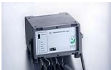
Thermal Comfort Data Logger used by Thermal Environmental Comfort Technicians to measure the six metrics.
